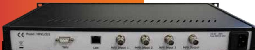
At the back you can find the connections for the MPX inputs and the network connection. There is also a 9 pin D connector with the text "Tally"
